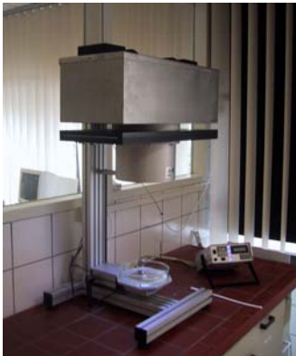
Figure 6: Collimated beam device for disinfection tests with UV irradiation
